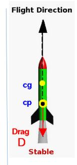
A stable rocket has its center of pressure (cp) behind the center of gravity (cg).
