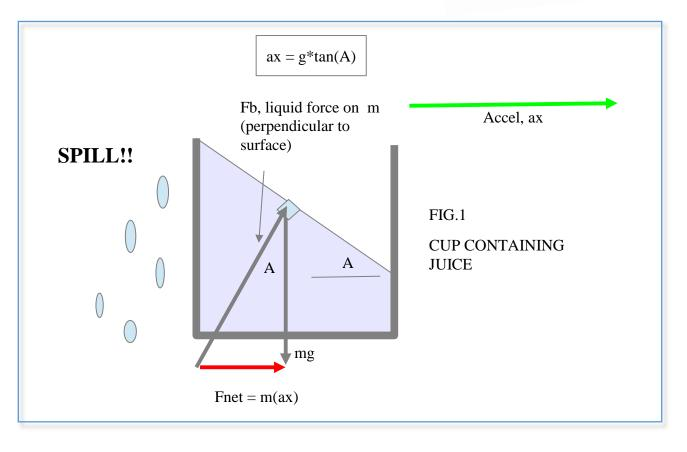
By contrast, the SpillNot automatically tips the cup so that its top stays parallel to the juice surface (see FIG.2 on the next page). For example, if the juice surface tips to 30 degrees but the cup stays horizontal, the juice could spill. But if the cup also tips to 30 degrees, we get no spill!
