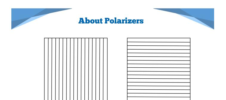
Only vertically oriented light waves may pass through the polarizing filter on the left. Only horizontally oriented light waves may pass through the filter on the right. If the filter on the left is placed on top of the filter on the right, no light will be able to pass through at all.
