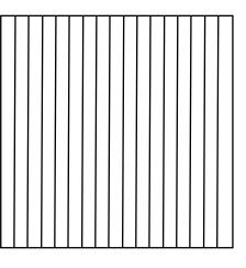
If the polarizing filters are aligned parallel to each other, light may pass freely through both filters. By placing transparent objects between two polarizing filters, it is possible to identify those materials which rotate polarized light!
