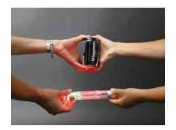
Next, give them a small **conductor** such as a paper clip, a key ring, or even a small metal staple. Students should place a finger on one electrode and—while holding the conductor you gave them—they should touch the other electrode with the conductor. The Energy Tube should
