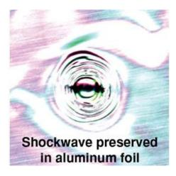
Repeat the experiment with a sheet of aluminum foil instead of paper. A number of concentric rings can be observed in the foil!
