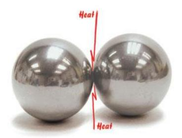
piece of ordinary paper! This amazing demonstration graphically illustrates the Law of Conservation of Energy as mechanical energy is transformed into heat energy. Although there are no flames, a charred hole appears along with the odor of burnt paper.
