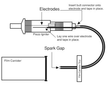
use heat shrink tubing over the electrical wires to make for a nice, neat looking apparatus.
