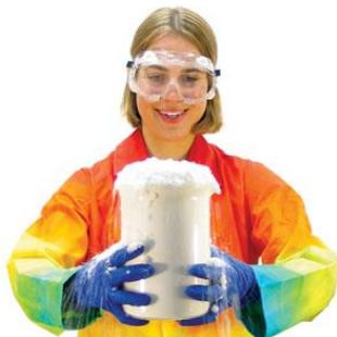
Instant Snow Polymer is a white granular powder which rapidly absorbs water. It will instantly absorb 40 times its original volume, producing a snow-like material.
