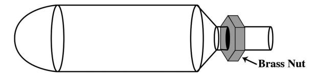
3. Fill each pipet bulb with colored water. Note that the bulbs must float when placed in a cup of water. Experiment with different amounts of water, making sure that the bulbs still float. Bulbs that float higher in a cup of water will make divers that are more difficult to sink.
