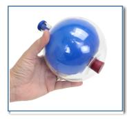
reduced and cannot act on the balloon. The glass in the Harbottle acts as a barrier between the atmosphere and the balloon.
