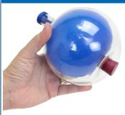
The balloon remains inflated without being knotted or tied because the pressure inside the balloon is greater than the pressure between the balloon and the Harbottle.
