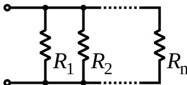
Fig. 2 Parallel circuit (of  $n$  resistors)
