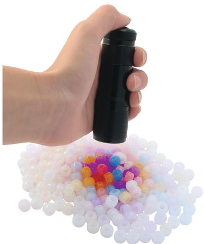
Although UV light is needed to excite the molecule to form the high-energy planar structure, heat from the surroundings provides the activation energy to change the molecule back to its colorless structure. If colored beads are placed in liquid nitrogen, they will not have enough activation energy to return to the colorless form. The UV detecting beads remain one of the least expensive qualitative UV detectors available today. They cycle back and forth thousands of times.
