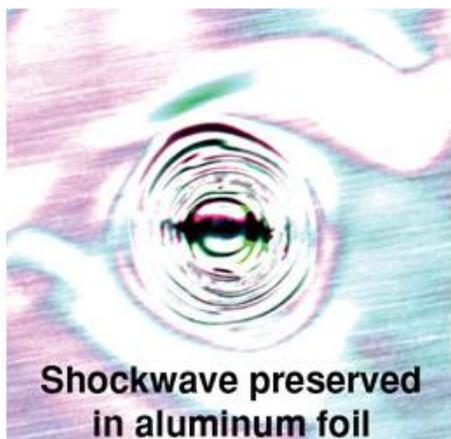
Repeat the experiment with a sheet of aluminum foil instead of paper. A number of concentric rings can be observed in the foil!
