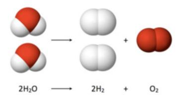
current through the fuel cell when it's filled with water causes the water to split into hydrogen and oxygen. If the fuel cell is attached to a motor while oxygen and hydrogen are present, it will combine them into water and produce an electric current that powers the motor. To learn more about how a hydrogen fuel cell works, click here.
