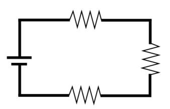
Fig. 1 Series circuit (with 3 resistors)
