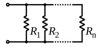
*Fig. 2 Parallel circuit (of n resistors)*
